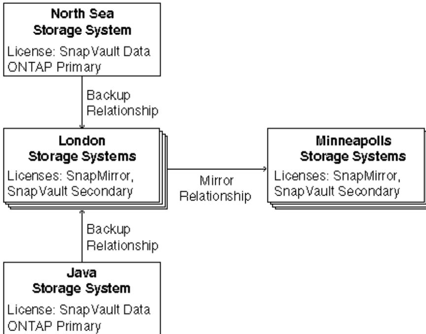
**North Sea storage system** This storage system stores the North Sea seismic test data in need of protection, so enable the SnapVault Data ONTAP Primary license on this system.
